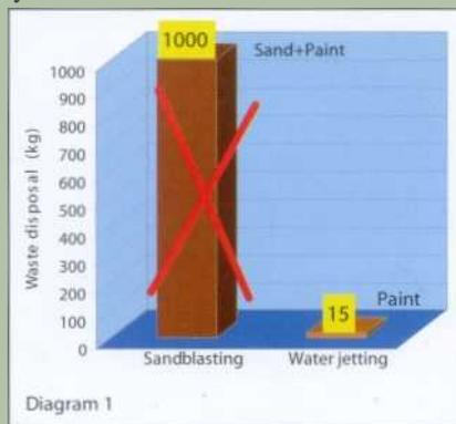
*Enormous sand volumes are consumed to remove paint when sand blasting. This problem waste can be avoided if sand blasting is replaced by water jetting.*
